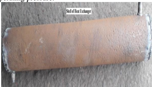
Shell of Heat Exchanger.
