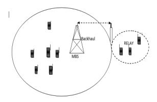
Figure 1: User Equipment Relays
