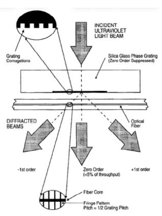
Figure 1: Bragg grating fabrication apparatus based on a zero-order nulled diffraction phase mask [1]
