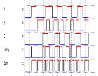
Figure 4 Overall Timing Diagram of DSCH Full Adder Design
