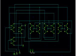
Figure 2 Implemented Design of Proposed Full Adder Module
