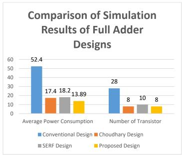
Figure 7 Chart shows the Comparison of Simulation Results of Full Adder Designs
