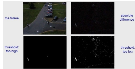
Frame difference results with Thresholds set at high and low.
